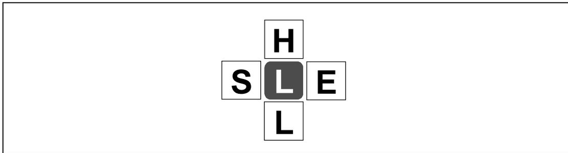
**Figure 1** SHEL Model. Source: Edwards, 1972 (as referenced in ICAO Human Factors Digest No 1, Circular 216 (1989))
