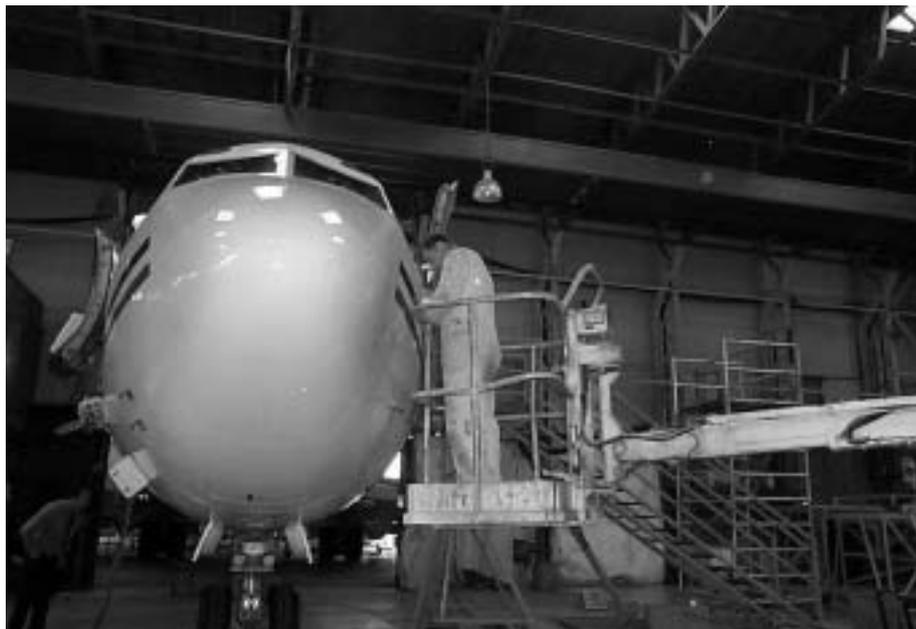
**Photograph E** Mobile access platforms, such as a "Cherry Picker", must be stable in use
