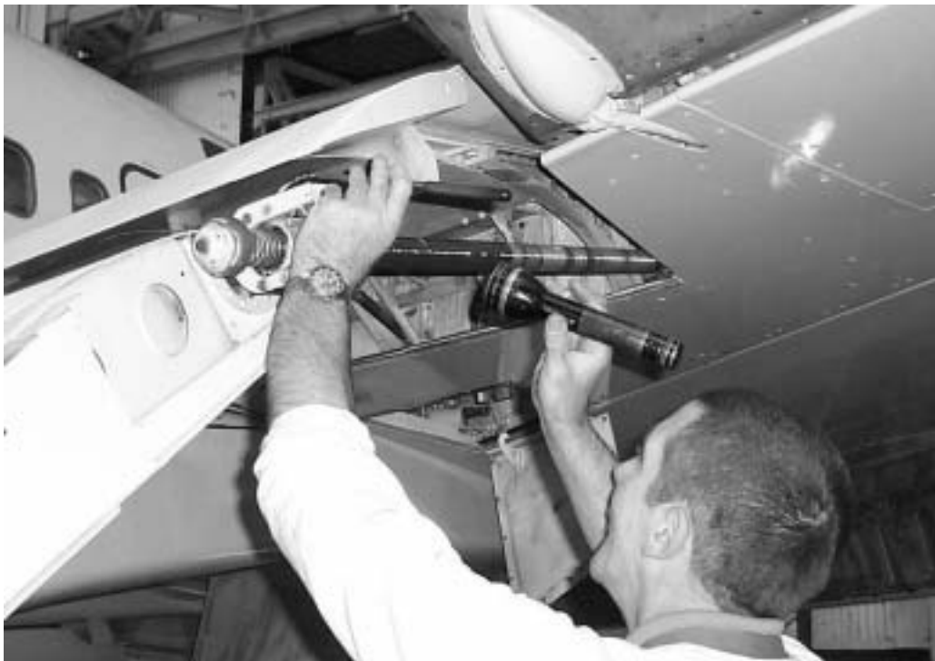
Photograph C Use of artificial lighting to supplement the ambient illumination in a hangar
