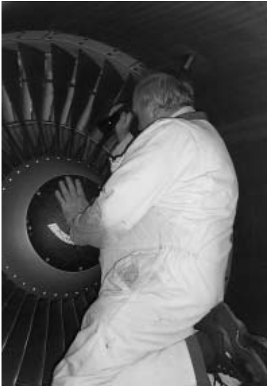
Photograph H An engineer making a visual inspection of engine fan blades
