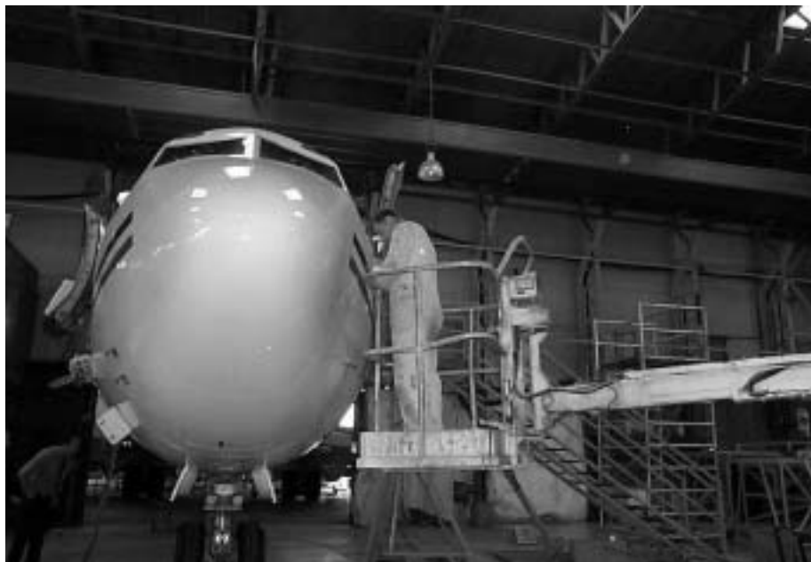
Photograph E Mobile access platforms, such as a "Cherry Picker", must be stable in use
